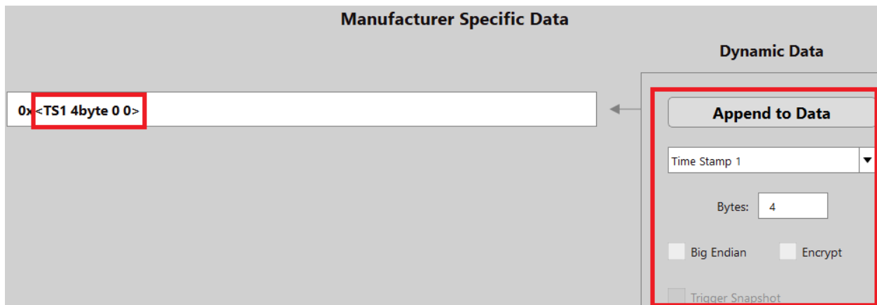
Figure 18 : Including the nonce counter in the advertising data: advertising counter
